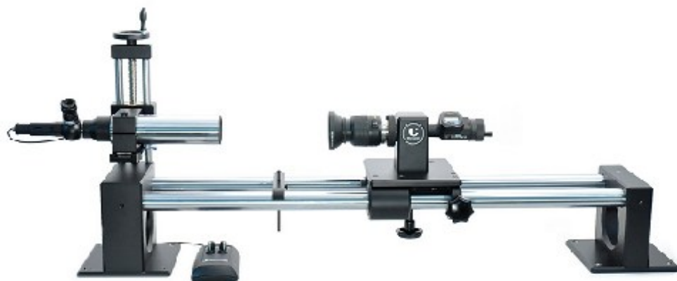
Autoreflex Collimator , measuring with a Siemens star
